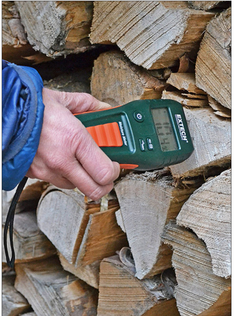
photo by Vanessa Fournier A patron of the Jeudevine Library in Hardwick uses the handheld wood moisture meter to check the moisture content of firewood. The device can be loaned out from the library for a week at a time. Twenty percent or less moisture content is suitable for burning. Vermont Agency of Natural Resources Department of Environmental Conservation in partnership with 48 libraries throughout the state have made the device available.
