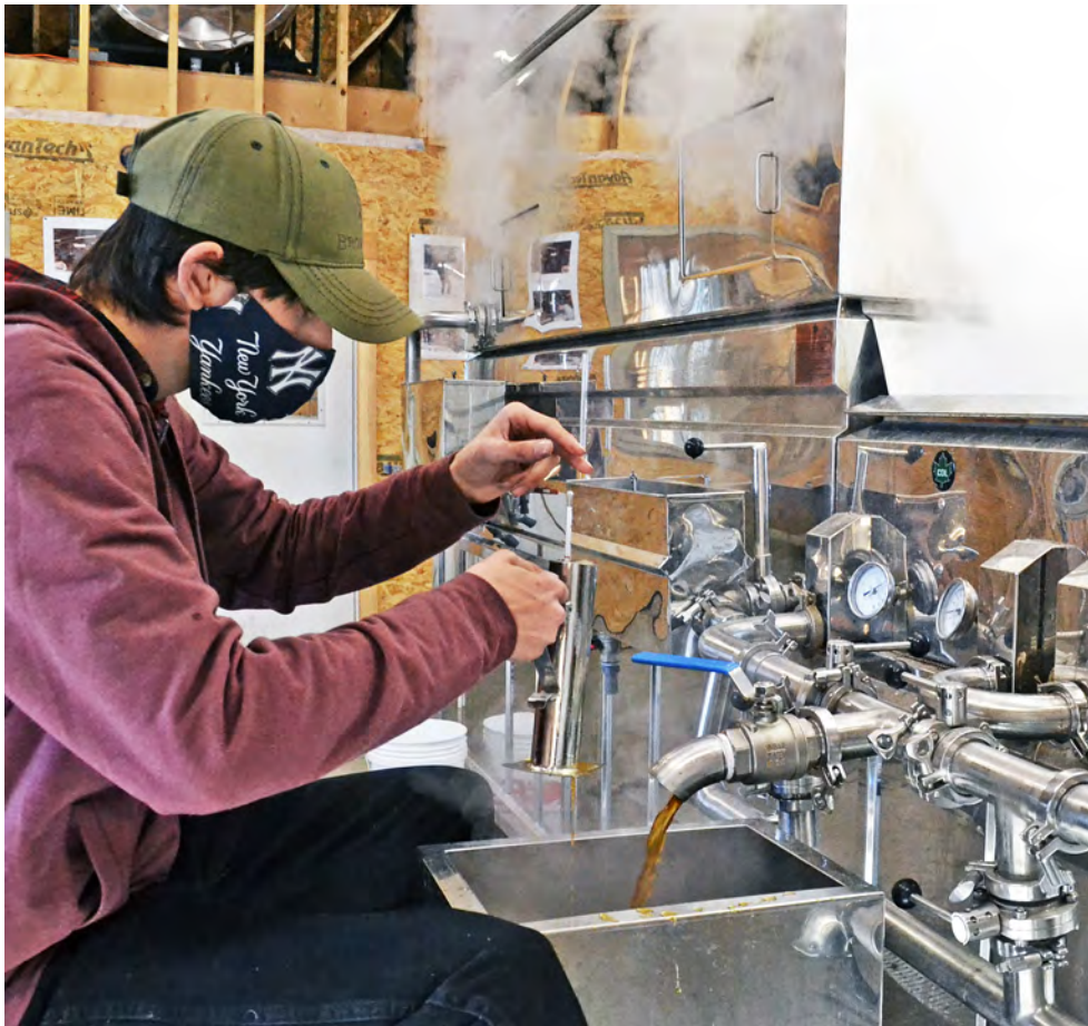
photo by Vanessa Fournier Green Mountain Technology & Career Center forestry student Tucker Baker checks the density of the syrup with a hydrometer. On their first boil of the season on March 12 the students made 30 gallons of Amber Rich.
