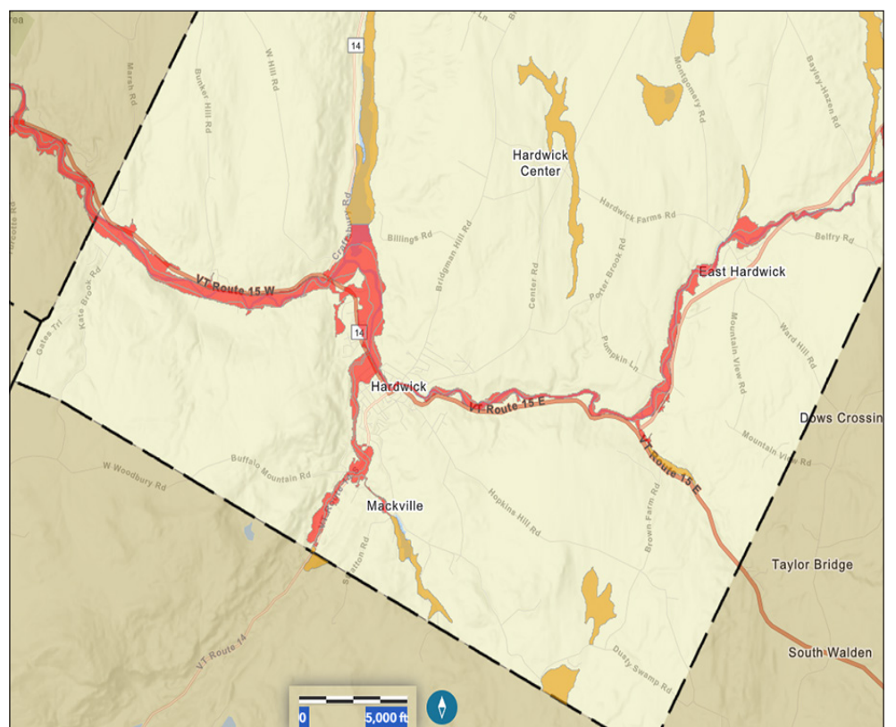
The Hardwick tax map with FEMA digitized flood hazard areas in red having a 1% annual chance of flooding. courtesy Town of Hardwick
